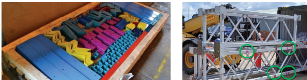
Figure 1: A crate of colored brackets and fixing connections of the off-site components of an industrial plant, which match to colored stickers positioned on the structural components (circled above) during the manufacturing process (Falmer 2016).
