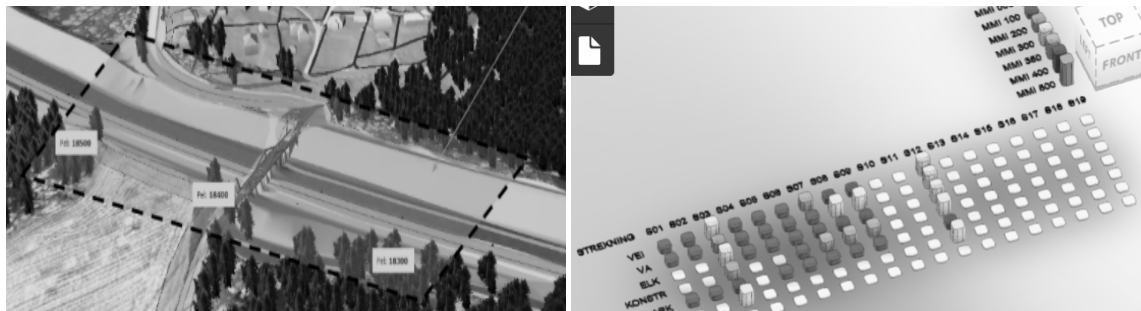
Figure 3: Example of section (left) and Visualization of MMI-levels, sections on x-axis, disciplines on y-axis (right)
